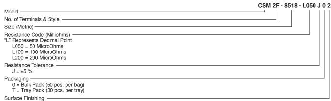
2 = Fully Tinned Terminals and Resistive Element
