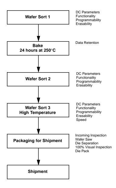
Figure 1. AMD KGD Product Test Flow
