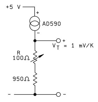
NOTE:  $V_S$  across device must remain constant or PSRR error must be included.
