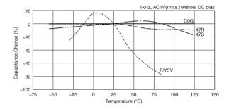
Capacitance - temperature characteristics
