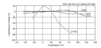
Capacitance - temperature characteristics
