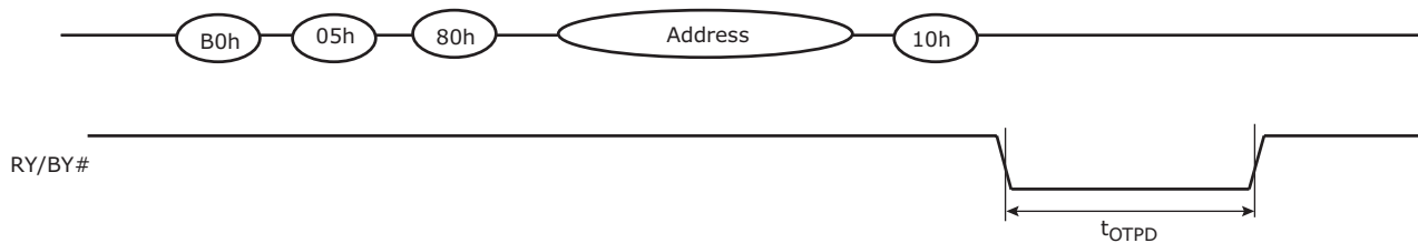
Figure 9.22 OTP Command (Page Protection Status) Timing Diagram
