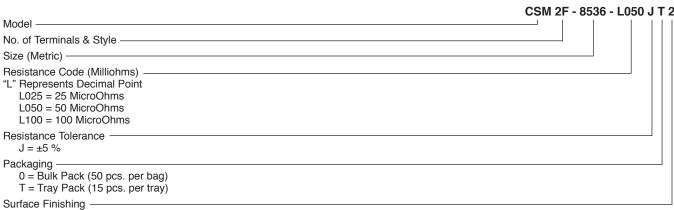
2 = Fully Tinned Terminals and Resistive Element
