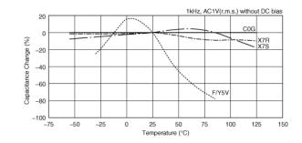
Capacitance - temperature characteristics
