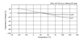
Capacitance - temperature characteristics
