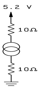
FIGURE 4. Radiation exposure circuit.
