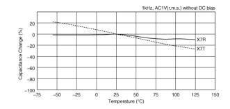
Capacitance - temperature characteristics
