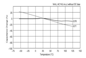
Capacitance - temperature characteristics
