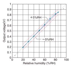
□ EXAMPLE OF THERMAL CHARACTERISTICS (TEMPERATURE DEPENDENCY) at Edc=5V, +15 to +35°C, 20% to 85%RH
