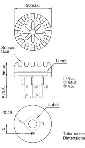
Tolerance:±0.2mm Dimensions in mm
