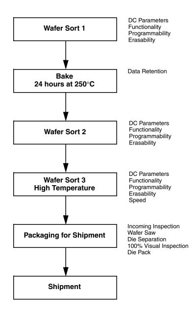
Figure 1. AMD KGD Product Test Flow
