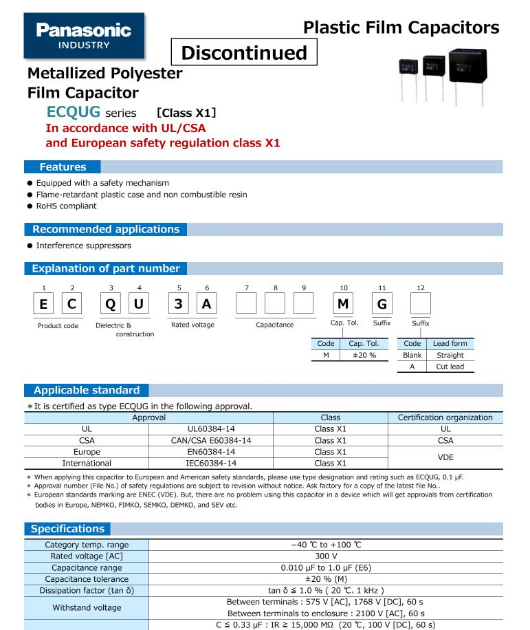
Insulation resistance (IR)C > 0.33 μF : IR ≥ 5,000 MΩ · μF (20 °C, 100 V [DC], 60 s)IR ≥ 2,000 MΩ (20 °C, 500 V [DC], 60 s)
