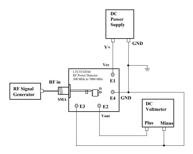
DC656A Demo Board Connection Diagram
