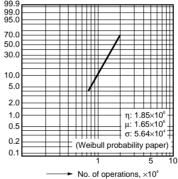
11.-(4)Electrical life (327 mA 24 V DC relay coil load) Tested sample: R-SD-24V, 5 pcs. Condition: HP2-DC24×6 pcs. in parallel, diode protector provided
