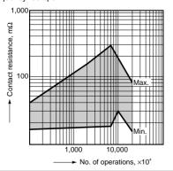
TEST RESULT No occurance of sticking was observed. Contact resistance: Fig. 1 R-SD-24V: 29 m $\Omega$  to 30.4 m $\Omega$
