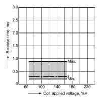
6. High frequency characteristics Tested sample: R-SD-24V Tested condition:
