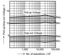
11.-(2) Electrical life Tested Sample: R-SD-24V, 10 pcs. Load: 60 mA 24 V DC resistive load
