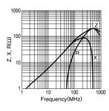
• TEST EQUIPMENT: RF IMPEDANCE ANALYZER YHP4191A
