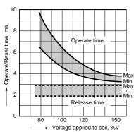
3.-(2) Set/Reset time (Latching) Sample: RK1-L-12V, RK1-L2-12V No. of samples: n = 12
