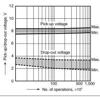
4.-(2) Mechanical life test (Latching) Sample: RK1-L2-12V
