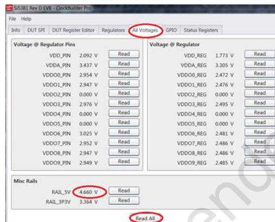
Figure 5.2. EVB GUI - Power Supply Check
