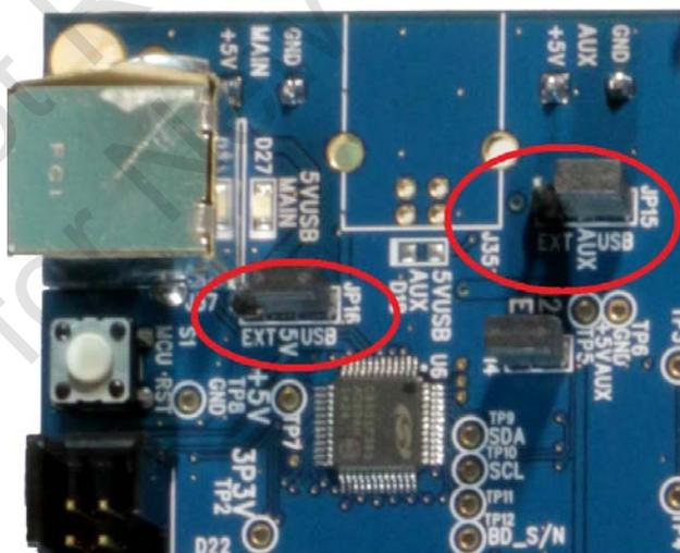
Figure 5.3. JP15-JP16 Standard Jumper Shunt Installation
