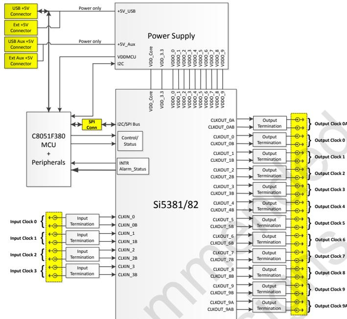
Figure 1.1. Functional Block Diagram of Si5381/82E-E-EB
