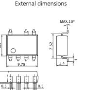
Terminal thickness: 0.25 General tolerance: ± 0.1
