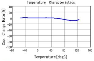
GRM188R72A332KA01 C-Temp. capchange, DCO.OV, AC1.C
