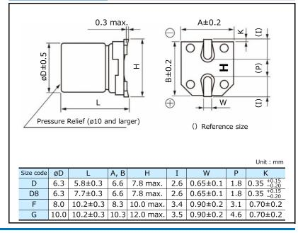
FKS-HF series (High temp. / Standard reflow)
