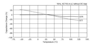
Capacitance - temperature characteristics
