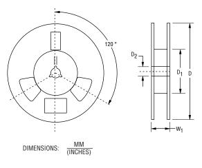
Devices are packed in accordance with EIA standard RS-481-A and specifications shown here.
