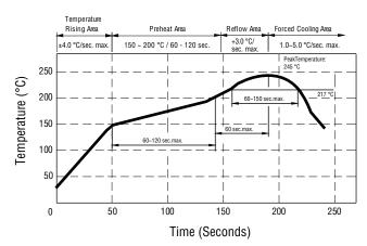
Peak Temperature: 245 ° ±5 °C max., 30 sec. max. Maximum Time Above 217 °C: 60~150 seconds
