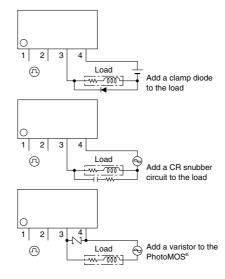
2) Even if spike voltages generated at the load are limited with a clamp diode or snubber circuit if the circuit wires are long, spike voltages will occur by inductance. Keep wires as short as possible to minimize inductance.
