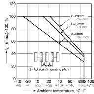
3. On resistance vs. ambient temperature characteristics
