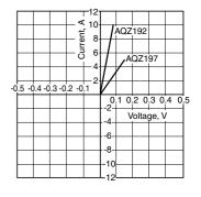
10. Leakage current vs. load voltage characteristics
