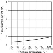
7. LED turn off current vs. ambient temperature characteristics Sample: All types
