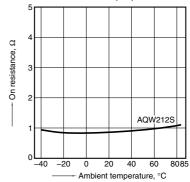
2.-(2) On resistance vs. ambient temperature characteristics
