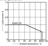
1.-(2) Load current vs. ambient temperature characteristics
