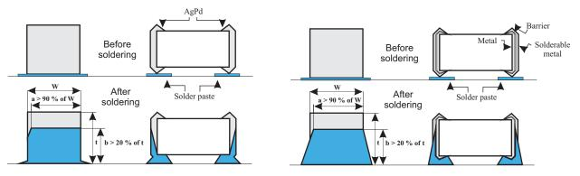
Fig. 5 Soldering Criterion in case of Wave and IR Reflow Pb-free Soldering
