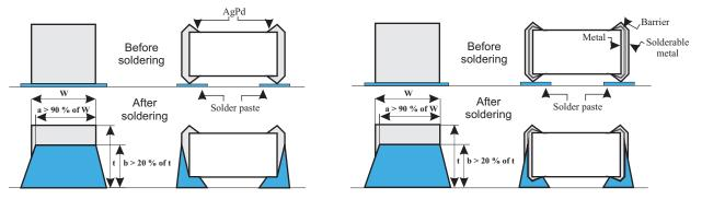
Fig. 4 Soldering Criterion in case of Wave and IR Reflow Pb-containing Soldering
