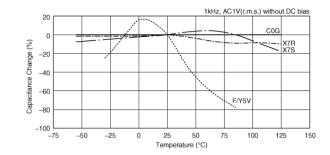
Capacitance - temperature characteristics
