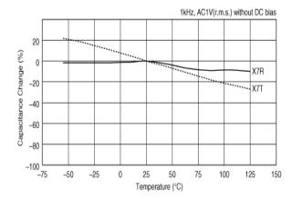
Capacitance - temperature characteristics
