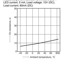
2. On resistance vs. ambient temperature
