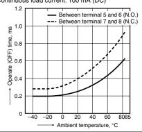
4. Reverse time vs. ambient temperature characteristics
