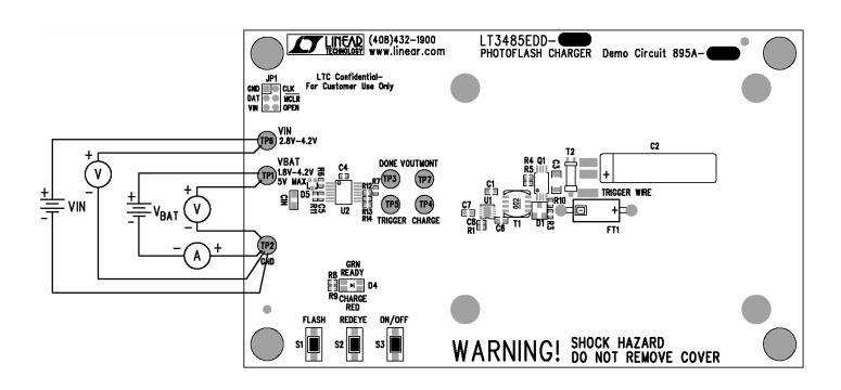
Figure 1. Proper Measurement Equipment Setup
