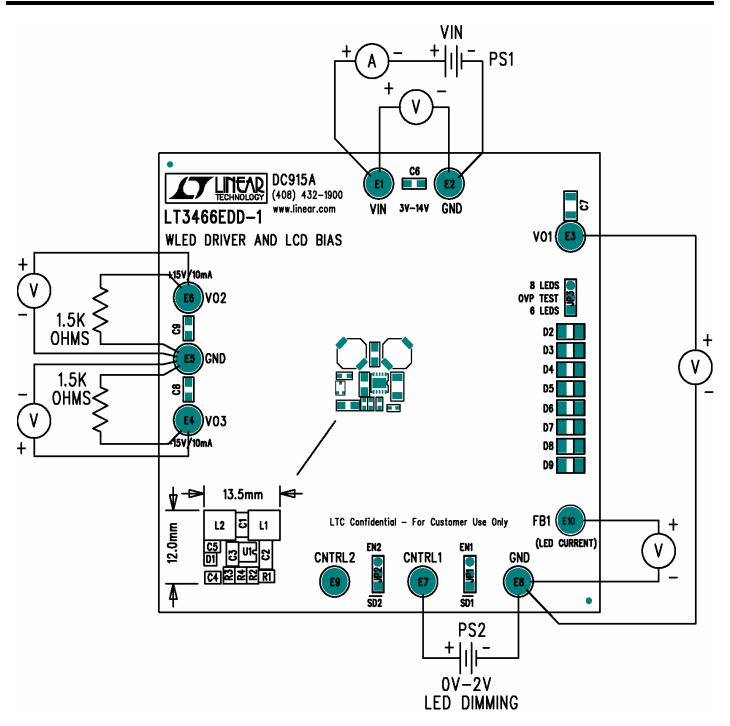
Figure 1. Test Connection Diagram
