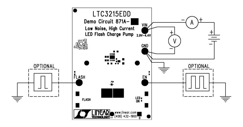
Figure 1. Proper Measurement Equipment Setup
