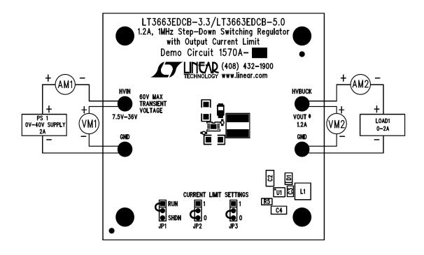
**Figure 1: Proper Measurement Equipment Setup**
