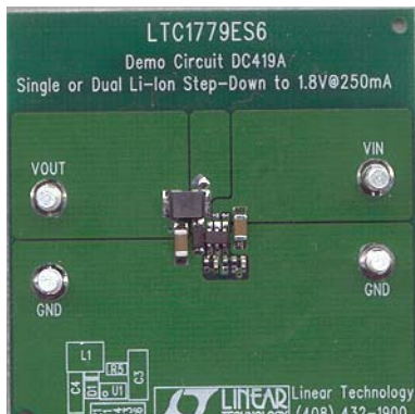
Figure 1... Quick Start connections for DC419A.
