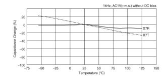
Capacitance - temperature characteristics
