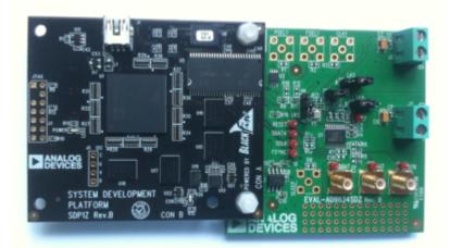
The AD9834 is a 75 MHz, low power DDS device capable of producing high performance sine and triangular outputs. It also has an on-board comparator that allows a square wave to be produced for clock generation. Consuming only 20 mW of power at 3 V makes the AD9834 an ideal candidate for power-sensitive applications.
