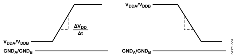
Figure 14. Transient Immunity Waveforms—Output Supplies
