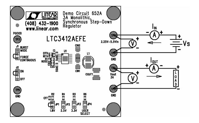
Figure 1. Proper Measurement Equipment Setup
