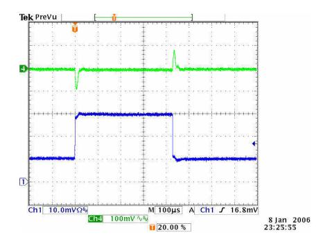
Figure 3. Load Step Response V<sub>IN</sub> = 3.3V, V<sub>OUT</sub> = 2.5V, 2A Load Step Trace 1: Output Voltage (100mV/div AC) Trace 2: Output Current (1A/div)
