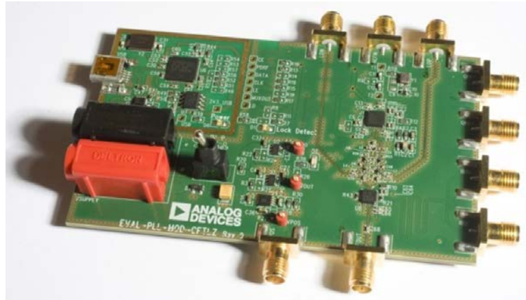
Figure 2. Evaluation Board for CN-0285 Direct Conversion Transmitter
