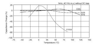
Capacitance - temperature characteristics
