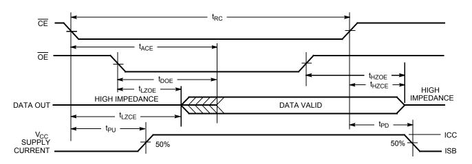
Notes: 10. Device is continuously selected.  $\overline{OE}$ ,  $\overline{CE} = V_{IL}$ . 11. WE is HIGH for read cycle. 12. Address valid prior to or coincident with  $\overline{CE}$  transition LOW.
