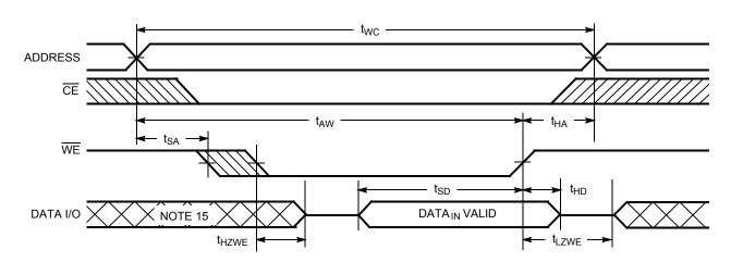
Notes: 13. Data I/O is high impedance if  $\overline{OE} = V_{|H...}$ 14. If  $\overline{CE}$  goes HIGH simultaneously with WE HIGH, the output remains in a high-impedance state. 15. During this period, the I/Os are in the output state and input signals should not be applied.
