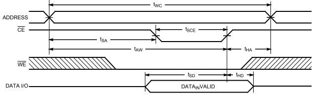
Write Cycle No. 3 ( $\overline{\text{WE}}$  Controlled,  $\overline{\text{OE}}$  LOW)<sup>[9, 14]</sup>
