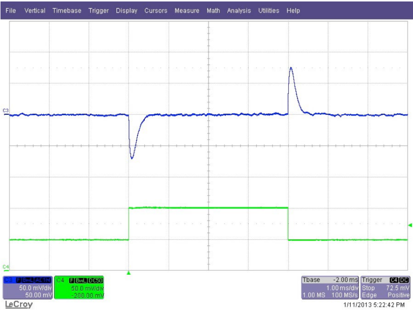
Figure 2. DC1922A Step Response
