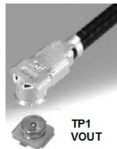
Figure 3b. Technique for Measuring Output Ripple and Step Response with a Low Inductance Connector (Not Supplied)
