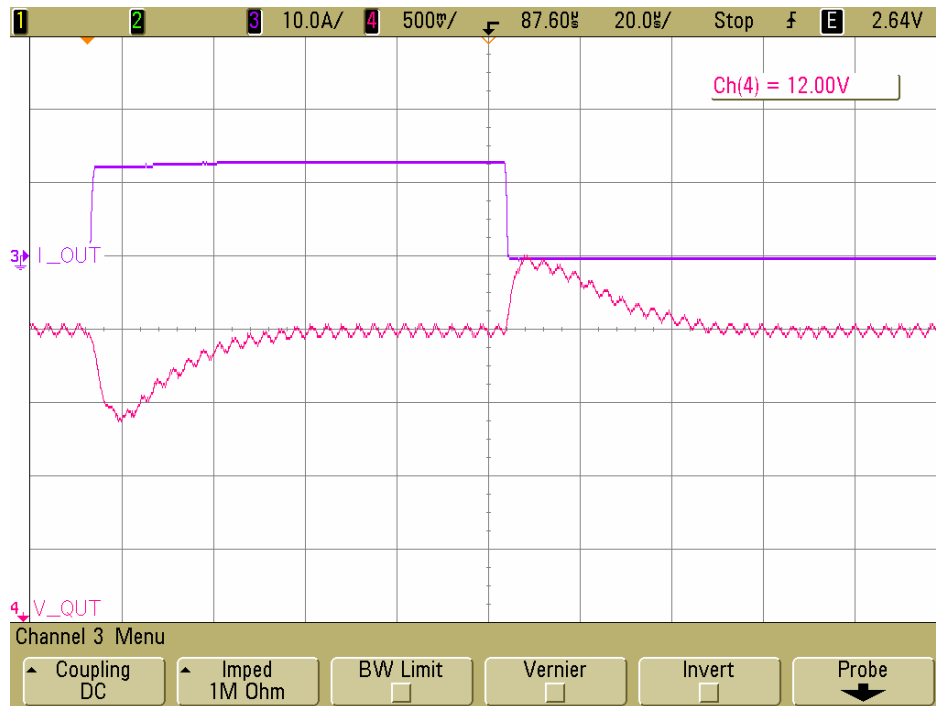
Figure 5. Load Transient Response (48Vin, 0A to 12Aout)
