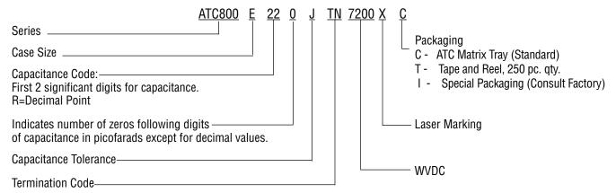
The above part number refers to a 800 E Series (case size E) 22 pF capacitor, J tolerance (±5%), 7200 WVDC, with TN termination (Tin Plated over Non-Magnetic Barrier Termination), laser marking and plastic Matrix Tray packaging.
