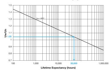
eg: rated voltage 1000V working voltage 1050V  $\rho = 1.05 \Rightarrow$  lifetime 50,000 hours @ 65°C hot spot temperature
